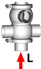
The valve opens from the top down by means of control air and closes bottom to top by means of spring tension without loss of product. In the closed setting, mix-proof separation of the media flowing in the upper and lower valve chambers is ensured by two independently closed valve plates. Any leaks occurring due to damaged valve plate seals are drained to the exterior without pressure via the leakage discharge (L).
